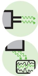
DC/DC-converters generate radiated interference as the result of high-frequency, periodic switching operations. The higher the switching frequencies and the steeper the leading or trailing edges of currents and voltages are, the greater will be the high-frequency component of the noise spectrum.
