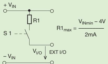
S1 closed  $\hat{=}$  unit off ( $V_{I/O} \geq 4\text{V}$ )
