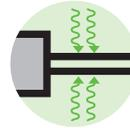
Bursts occur during switching operations, e.g. disconnecting inductive loads and bounce of relay contacts, in all electrical power supply systems. The burst test is intended to guarantee that the function of electrical loads is not impaired on a sustained basis as the result of these extremely brief voltage peaks. The standard demands: Assessment criterion B. Kniel DC/DC converters comply with evaluation criterion A.
