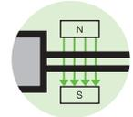
In the frequency range between 50Hz and 60Hz the device is applied with 30A/m. There must be no interference. Kniel DC/DC converters comply with assessment criterion A.
