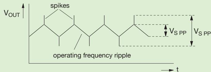
Fig. 2 Voltage variation of the output when subject to a defined sudden load variation
