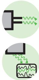
In primary switched power supplies radiated noise is generated by high-frequency, periodic switching operations. The higher the switching frequencies and the steeper the rising or falling edges of current and voltage are, the higher will be the high-frequency share of the noise spectrum.
