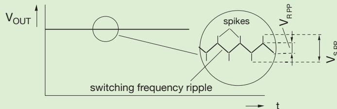
Fig. 2 Voltage change at the output in the event of a defined sudden load change
