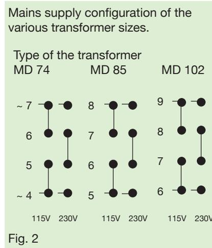
Note: The type of the transformer can be recognised by the configuration of the pins.
