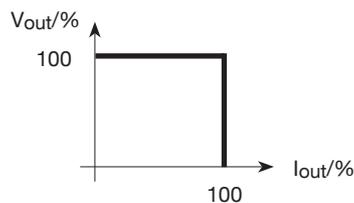
Fig. 3 VI-characteristic curve
