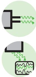
In Low Emission units radiated noise is generated by high-frequency, periodic switching operations.
