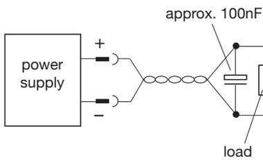
In the case of a power supply with an output voltage above 60Vdc, the user must ensure that the output and load connections as well as the measurement configuration cannot be touched!
