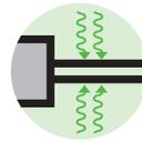
Fast transient bursts occur during switching operations, e.g. disconnecting inductive loads and bounce of relay contacts, in all electrical power supply systems.
