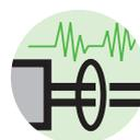
In the frequency band 150kHz to 80MHz, the equipment is subject to modulated fields which induce noise voltages of 10V in the supply lead.
