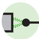
This test verifies the immunity to electrostatic discharge as may occur from the operator's body when touching the equipment. Static discharges as can arise between different objects are also covered with this test.
