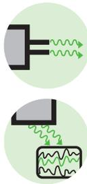
In primary switched power supplies radiated noise is generated by high-frequency, periodic switching operations. The higher the switching frequencies and the steeper the rising or falling edges of current and voltage are, the higher will be the high-frequency share of the noise spectrum.
