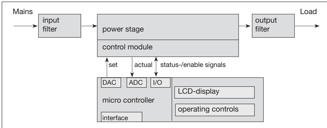
The unit is powered from a three-phase power system without neutral conductor. The internal supply voltage is generated via the input filter. This voltage is used, in turn, to power the output stage. Actual conversion to an electrically isolated output voltage that is supplied to the load terminals via the output filter occurs in this output stage.
