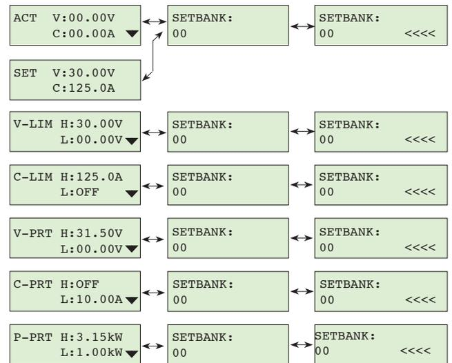
**NOTE:** The selected memory bank is always active, i.e. its settings are assigned directly to the device output and only these settings can be edited. Settings from inactive memory banks cannot be edited.
