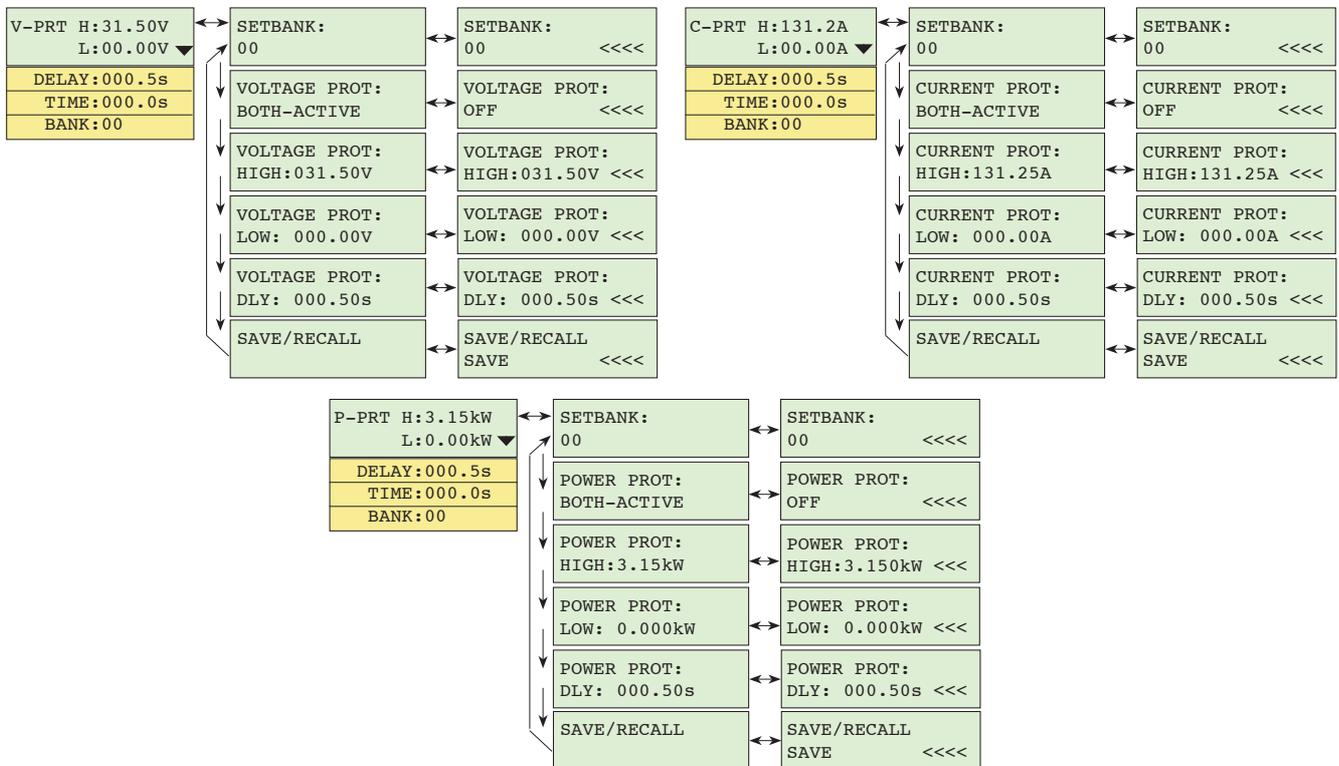
**NOTE:** The currently elapsed time since occurrence of the error state is indicated in the fourth line with "TIME" in the case of the Protection Status displays. This allows you to estimate the time through to deactivation of the device.
