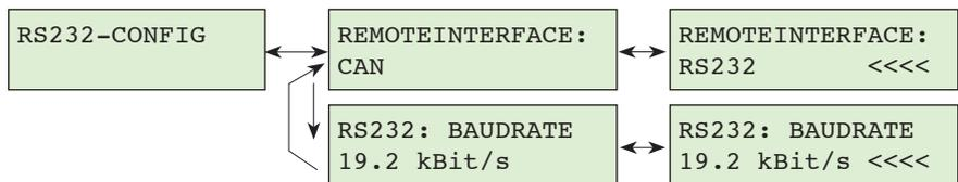
**NOTE:** The required interface is selected with "REMOTEINTERFACE". Only one interface may be used at any one time.
