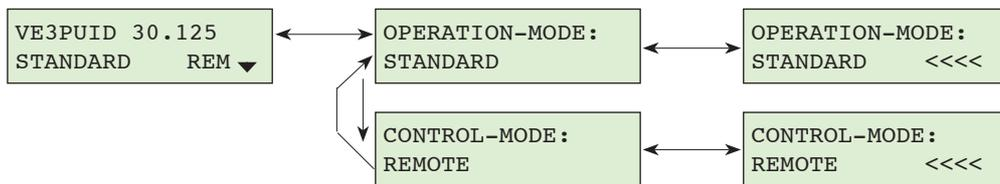
**NOTE:** The modes can be changed in any operating mode and any control mode. The output may not be activated for reasons relating to safety.
