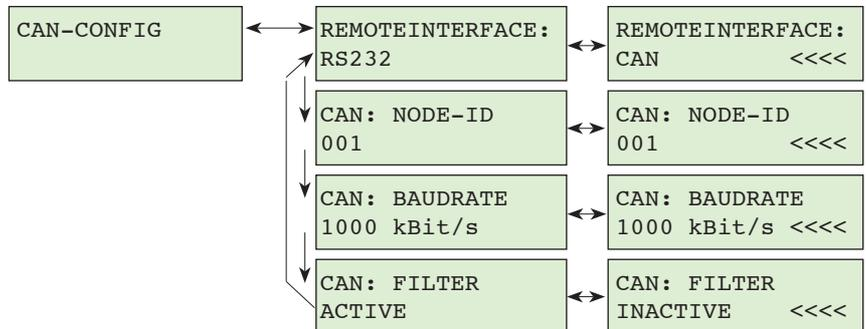
**NOTE:** The required interface can be selected with "REMOTEINTERFACE". Only one interface can be used at any one time.
