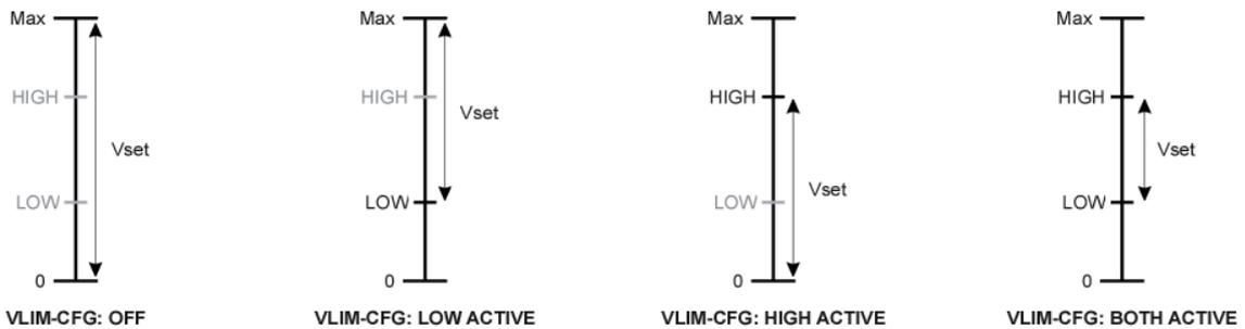
The setting range for the limit values is generally 0 to nominal value. In the case of configuration "BOTH ACTIVE", HIGH limits the setting range from LOW upwards and LOW limits the setting range from HIGH downwards.
