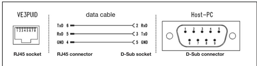
Data is transferred serially and bit-by-bit, whereby the transfer rate can be set optionally to 1200, 2400, 4800, 9600 or 19200 bit/s. 19200 bit/s is set in the condition as delivered.
