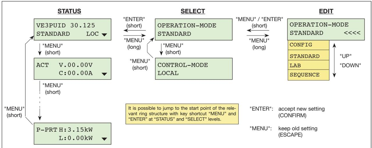
You can navigate within the menus with buttons "MENU" and "ENTER". The menu structure consists of three levels:
